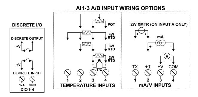
**Note:** TX power is only available on input A of each channel and is only enabled if the input channel is HLPRG with mA input configuration.
