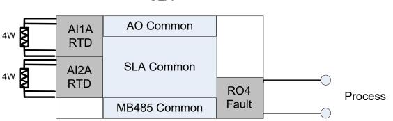
SLA with 1002 voting on RTDs wired to separate input channels. R4 Fault relay used as combined fault/trip relay, -3AO and –MB485 options are fitted but are NOT part of the safety function so only their common circuit fault factors need to be considered.
