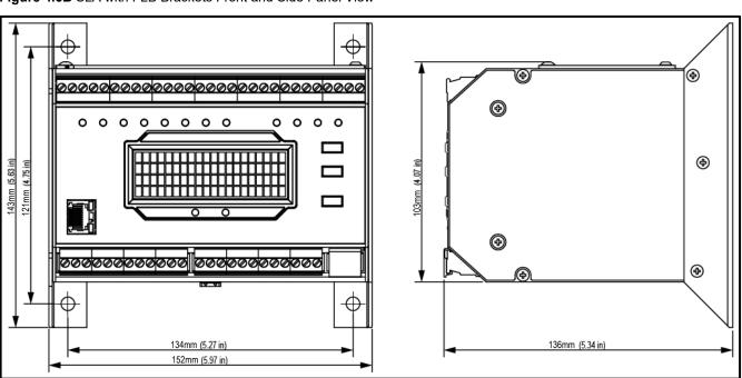
Figure 4.6B SLA with FLB Brackets Front and Side Panel View
