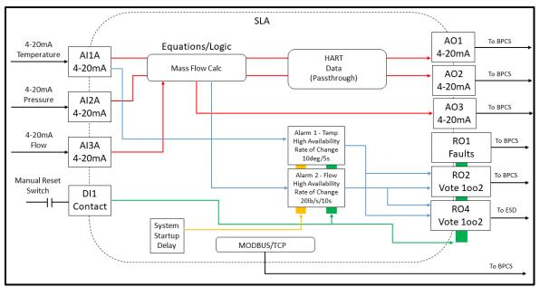
Figure 12.4 High Temperature and Flow SIS Programming Logic
