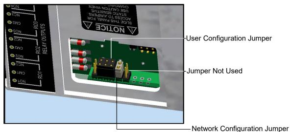
Figure 4.9 User and Network Configuration Security Jumpers in READ-ONLY position.
