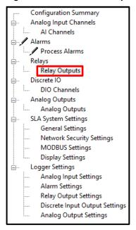
In the lefthand window of the SLA DTM, click on the + next to **Relays** and select **Relay Outputs** to configure.
