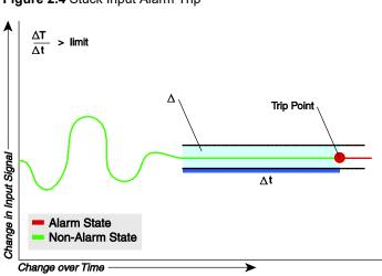
Figure 2.4 Stuck Input Alarm Trip
