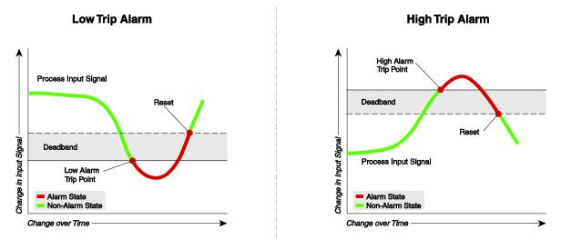
**Band Alarm** - The Band Alarm is a high and low trip alarm combined. It can be set using low and high trip points. Deadband can also be set for this alarm type.
