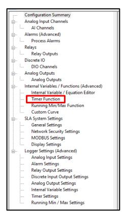
In the left window of the SLA DTM, click + next to **Internal Variables/Functions (Advanced)** and select **Timer Function** to configure the eight available Timers.
