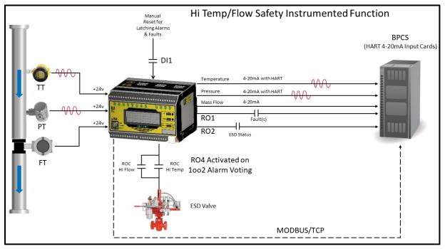
Figure 12.3 High Temperature and Flow Safety Instrumented System
