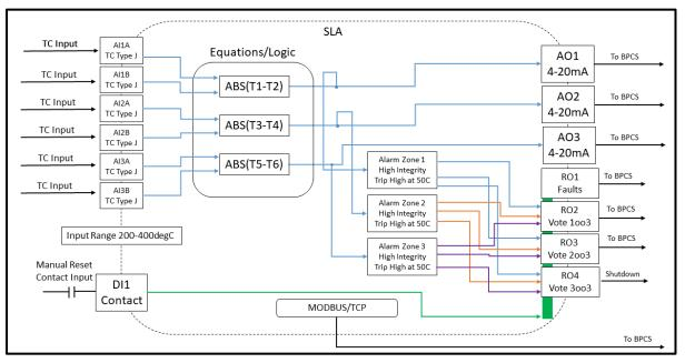
Figure 12.6 Temperature Alarm SIS Programming Logic
