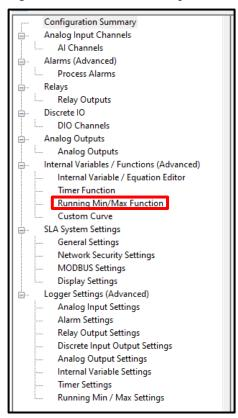
In the left window of the SLA DTM, click + next to **Internal Variables/Functions (Advanced)** and select **Running Min/Max Function** to configure the eight available Running Min/Max Functions.
