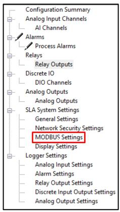
In the left window of the SLA DTM, click MODBUS Settings to configure MODBUS settings and RTU settings if –MB485 option is fitted.
