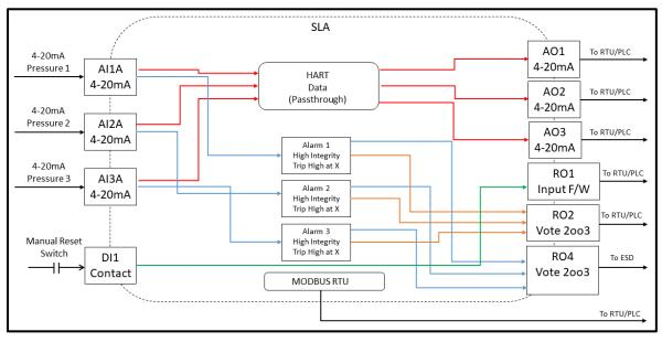
Figure 12.2 2003 Voting Shutdown System Programming Logic
