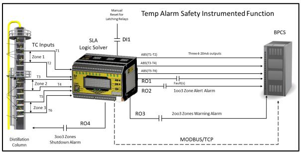
Figure 12.5 Temperature Alarm Safety Instrumented System
