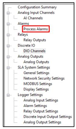
From the lefthand window of the SLA DTM, select Process Alarms under Alarms to configure up to 16 available alarms.
