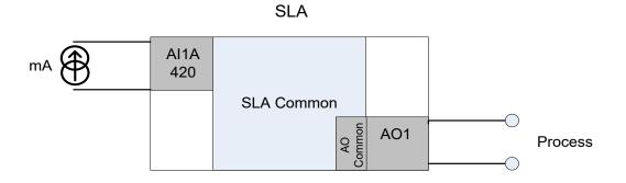
No Fault relay used, system faults are enabled on AO (this will not include hardware only detected faults).
