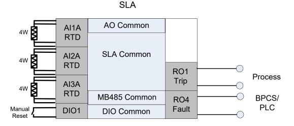
SLA with 2003 voting on RTDs wired to separate input channels. R1 is used as a process trip and R4 as a separate Fault relay to notify BPCS/PLC. DIO1 is used as a manual reset input. -3AO and -MB485 options are fitted but are NOT part of the safety function.
