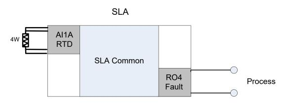
R4 Fault relay used as combined fault/trip relay.
