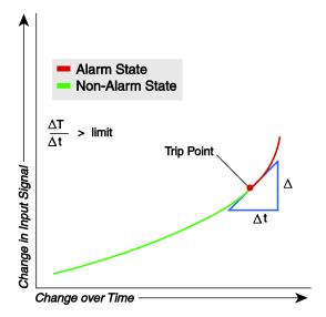
A Stuck Input Alarm also monitors an input for a change in value with respect to time (**Figure 2.4** below). The alarm is set to trip when the input does not change by a user-selected amount (Delta) over a user-selected time period (Delta Time). To set the correct value for delta and delta time, you need to understand the expected process variations to avoid false trips and the input signal noise and averaging filter settings to prevent missing stuck inputs.
