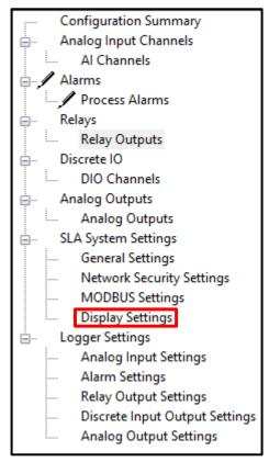
**Enable Display Auto Scroll**- When checked, SLA display will automatically scroll through selected parameters.
