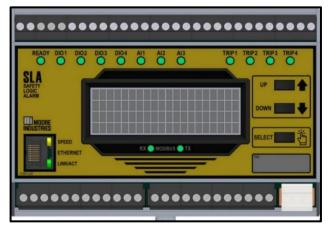
It is possible to toggle the Auto-scroll setting from the Display Settings screen. The change is not saved, therefore the Configuration ID is not affected. If the SLA is power-cycled, the last value set by the DTM will be applied.
