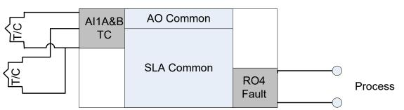
R4 Fault relay used as combined fault/trip relay; AO is used but is NOT part of the safety function.
