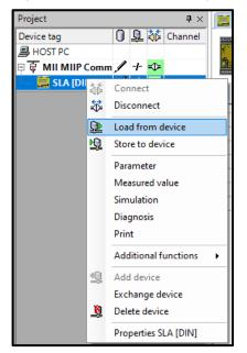
3. The SLA configuration is now uploaded and the **Configuration Summary** screen is ready to be displayed. Double click the SLA device in the project tree to view the Configuration Summary page.
