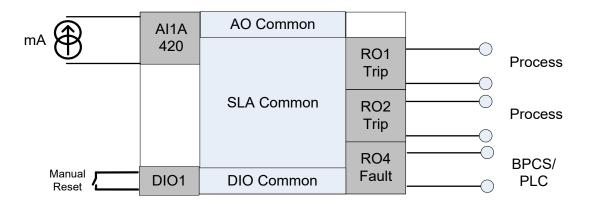
R1 and R2 are used as process trips and R4 as a separate Fault relay to notify BPCS/PLC. DIO1 is used as a manual reset input. -3AO option is fitted but is NOT part of the safety function.
